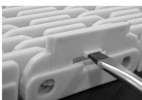
Remove open clip by pushing and turning screwdriver.
